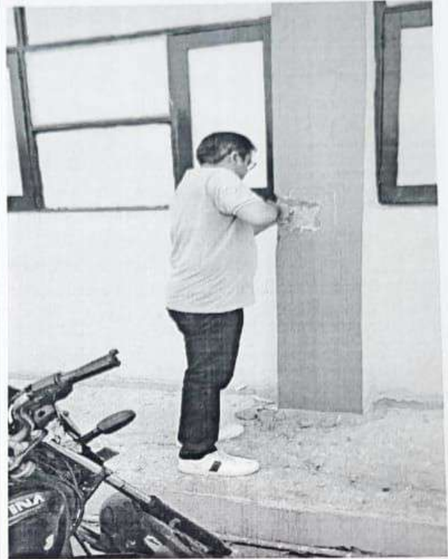
Rebound Hammer testing on RCC column locations at Sector 4Rohtak
